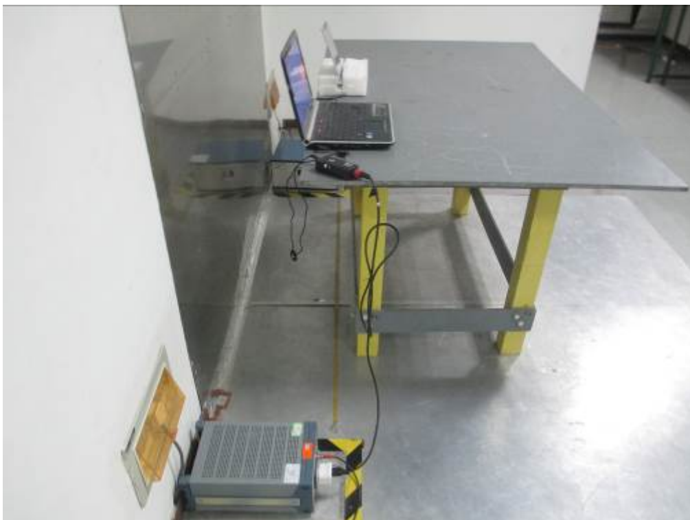
Conducted Emissions Test Setup Side View
