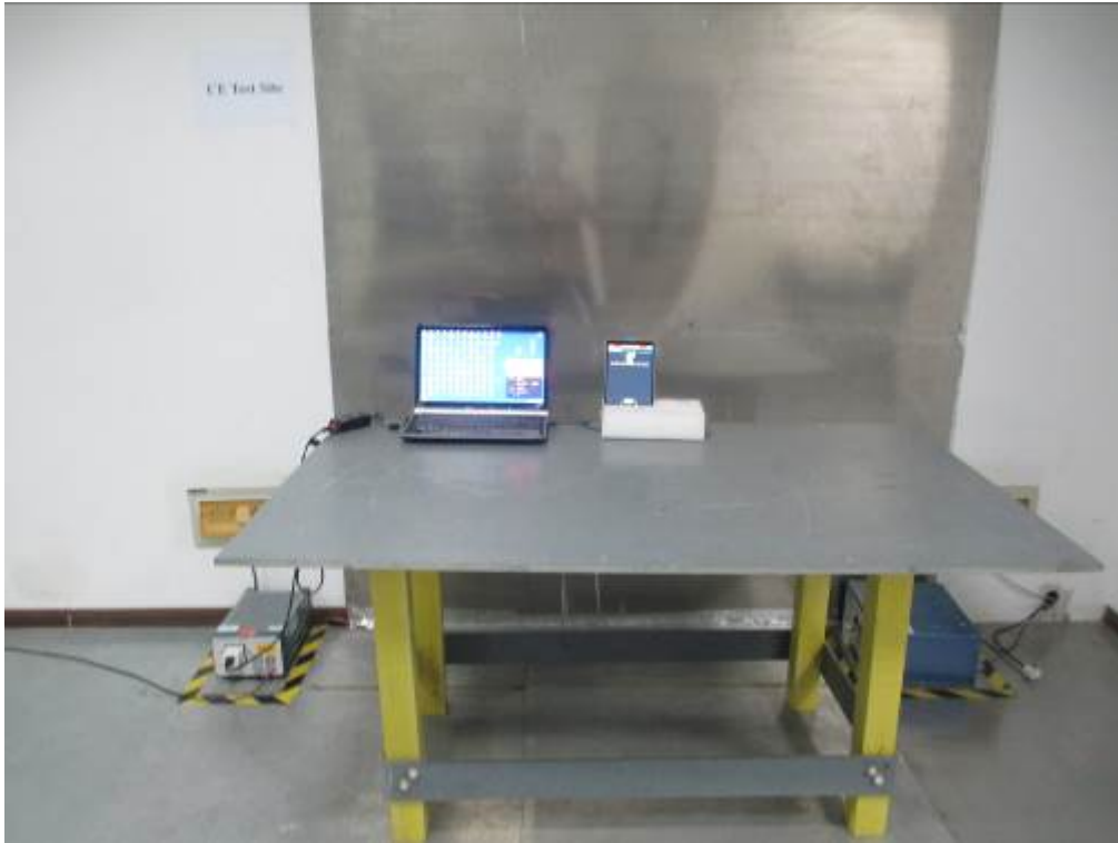
Conducted Emissions Test Setup Front View
