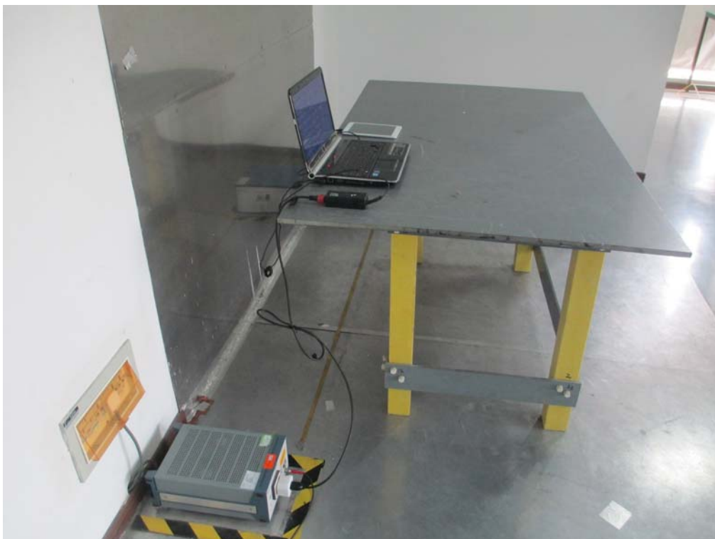
Conducted Emissions Test Setup – Side View
