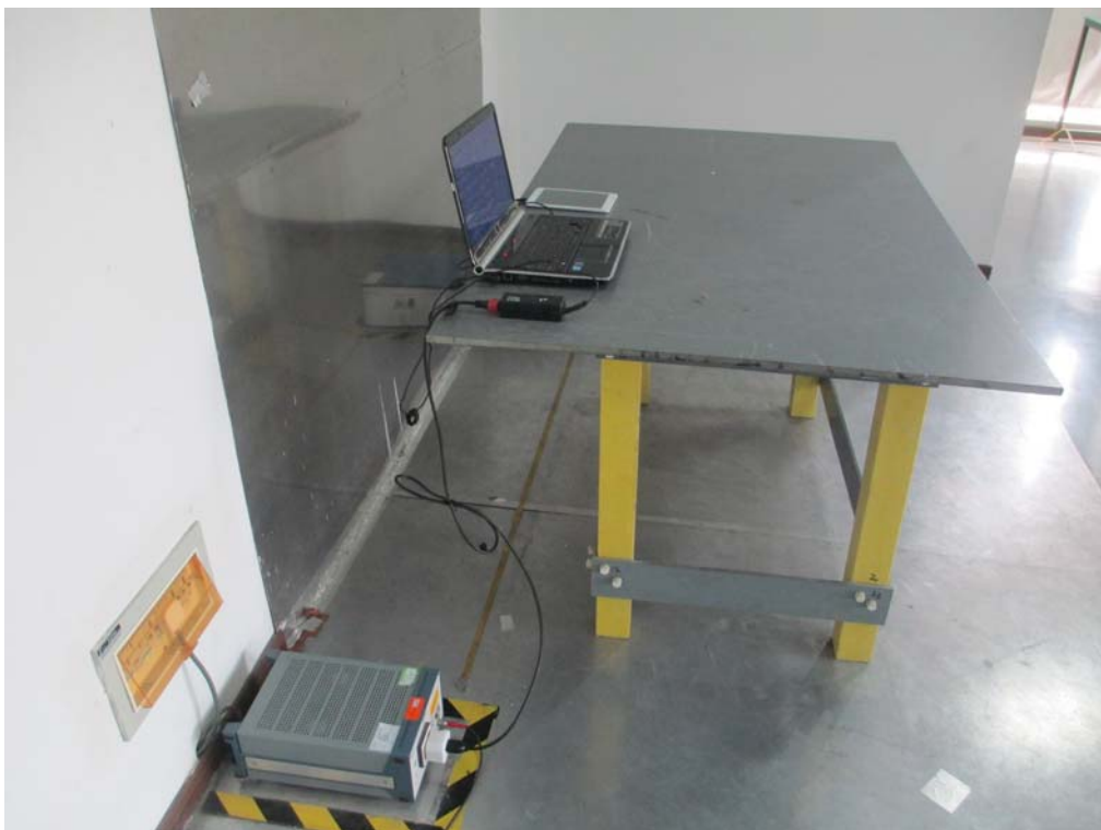
Conducted Emissions Test Setup – Side View
