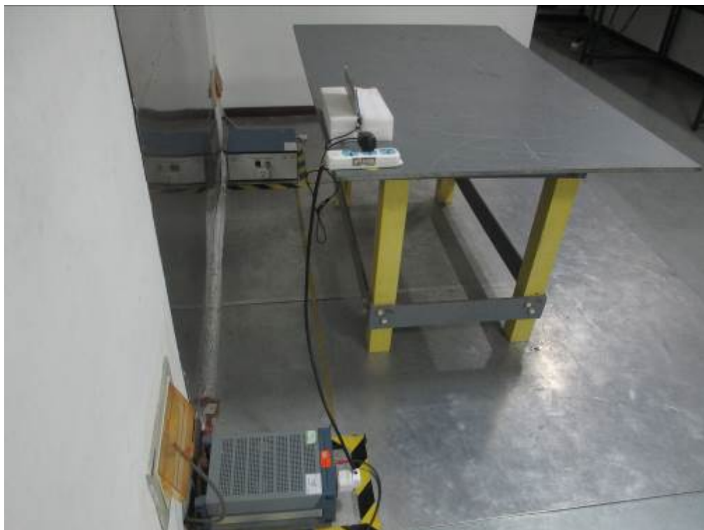
Conducted Emissions Test Setup – Side View
