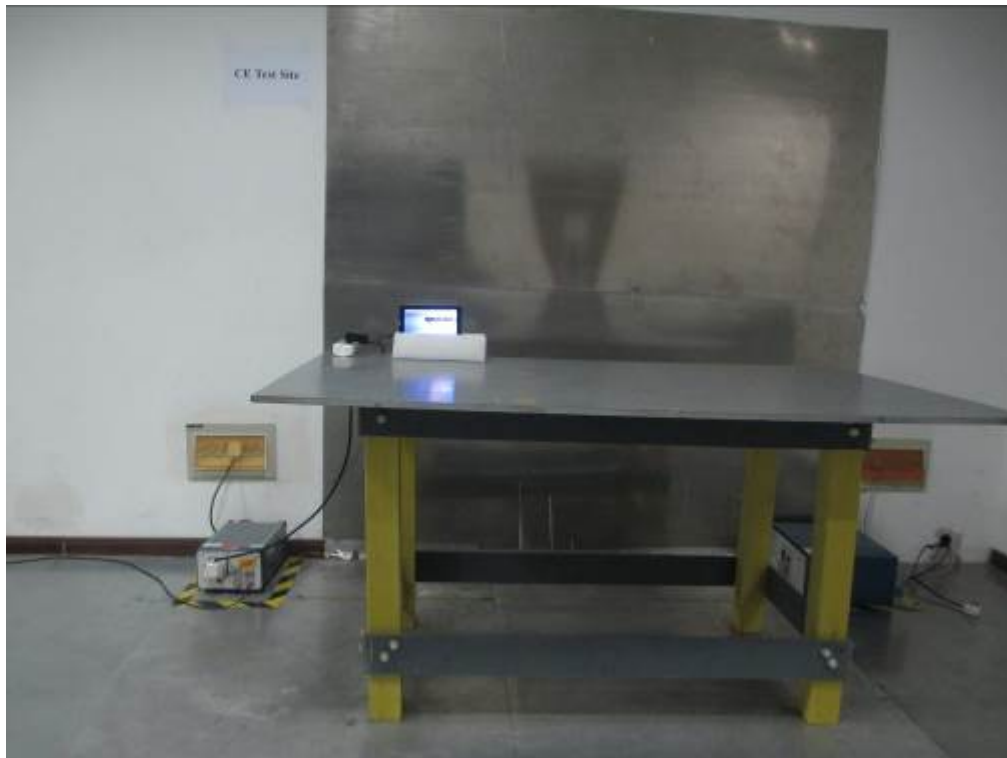
Conducted Emissions Test Setup – Front View
