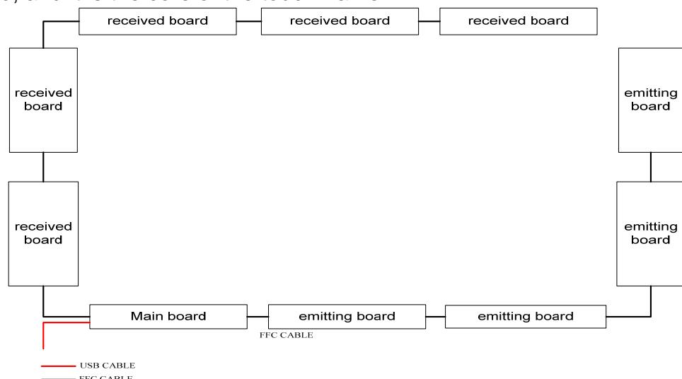
The two kinds of PCBA is standard modular. The different models have the same constructions, circuit diagram. The difference of these models is its size, is mainly reflected in the number of received board and emitting board in different.
