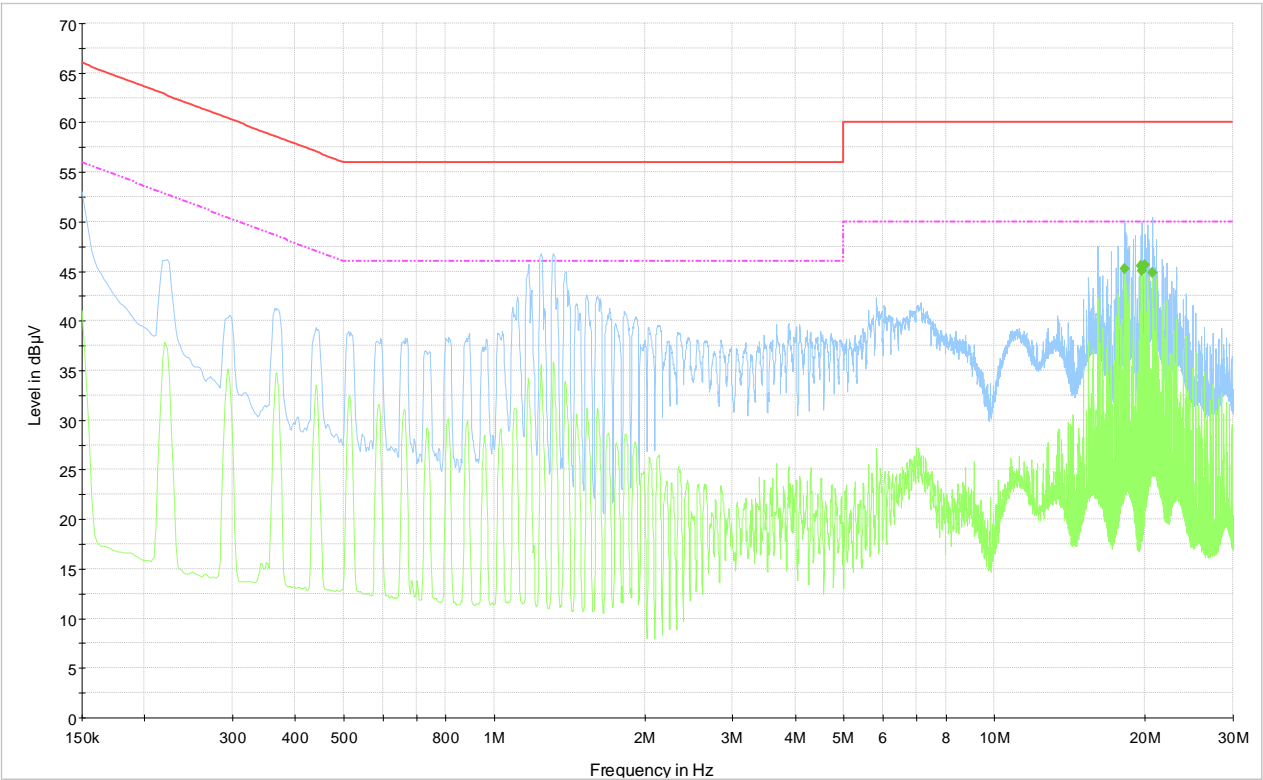
Plot 8.1-1: Conducted emissions on phase line
