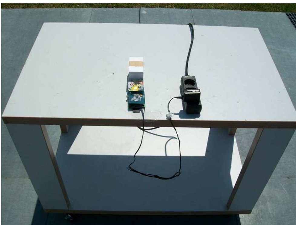
Figure 5: Radiated emission test – 9kHz to 30MHz (setup on a 10 m distance)
