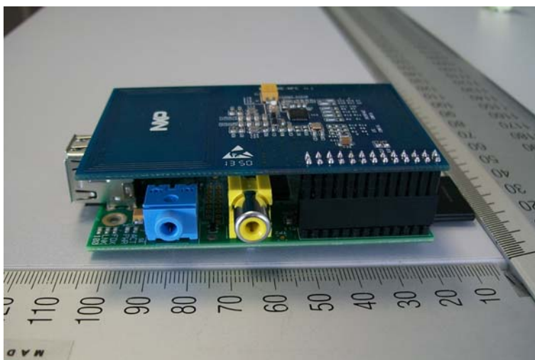
Photos of EXPLORE-NFC with Raspberry Pi
