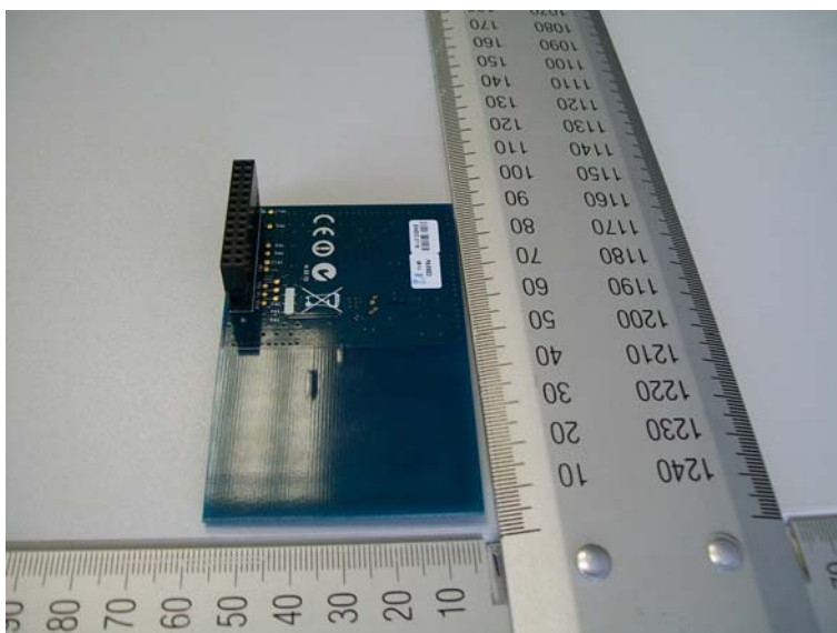
Photos of EXPLORE-NFC with Raspberry Pi
