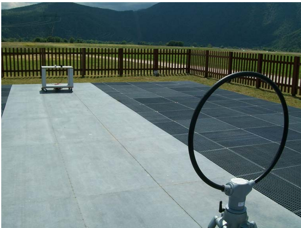
Figure 4: Radiated emission test – 9kHz to 30MHz (retested on a 10 m distance)
