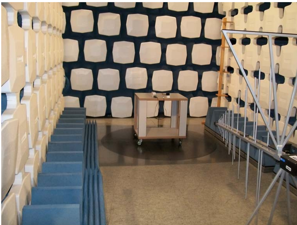
Figure 3: Radiated emission test – 30MHz to 1GHz
