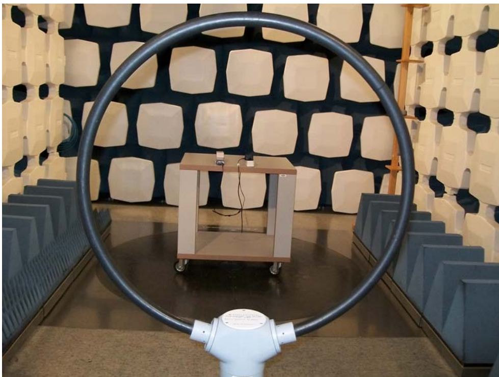
Figure 2: Radiated emission test – 9kHz to 30MHz
