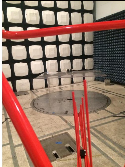
Photograph 1. Radiated Emission Set up, 30 MHz - 1 GHz
