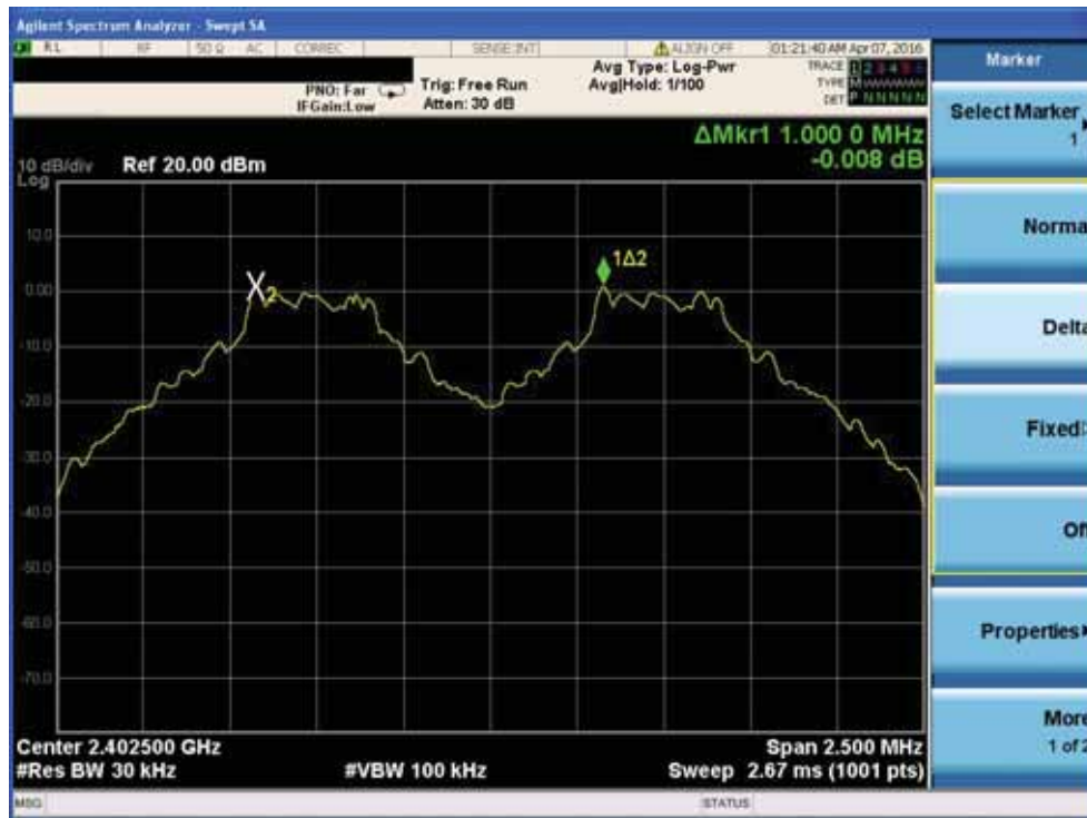
Channel Separation plot on channel 39-40
