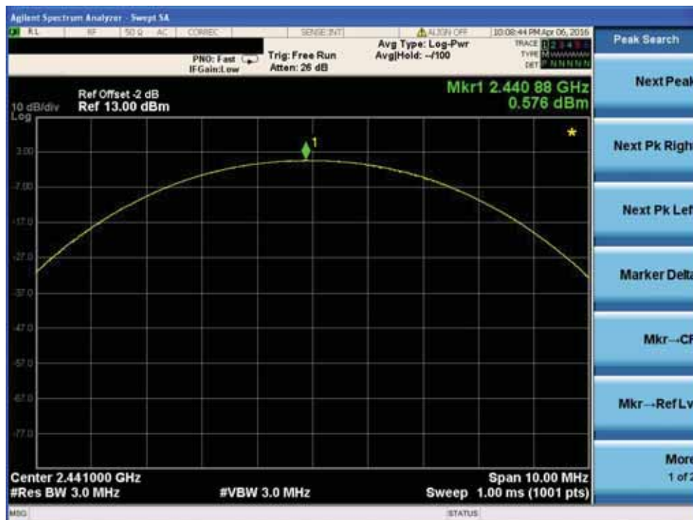
Peak output Power plot on channel 39
