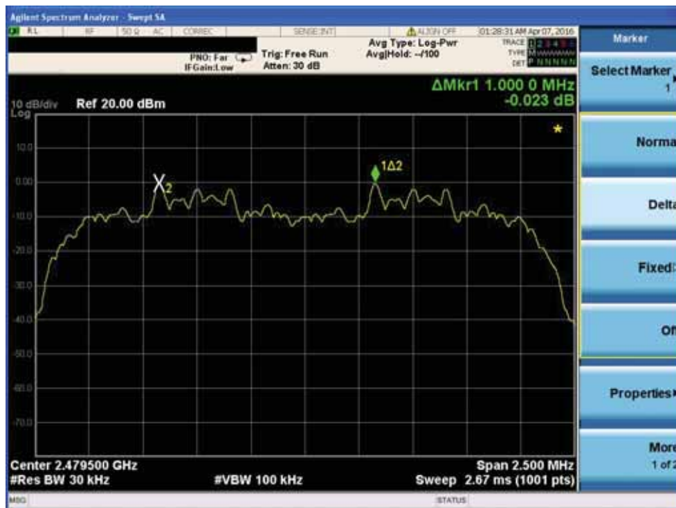
Channel Separation plot on channel 77-78
