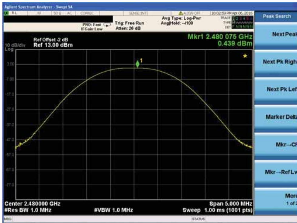
Peak output Power plot on channel 00
