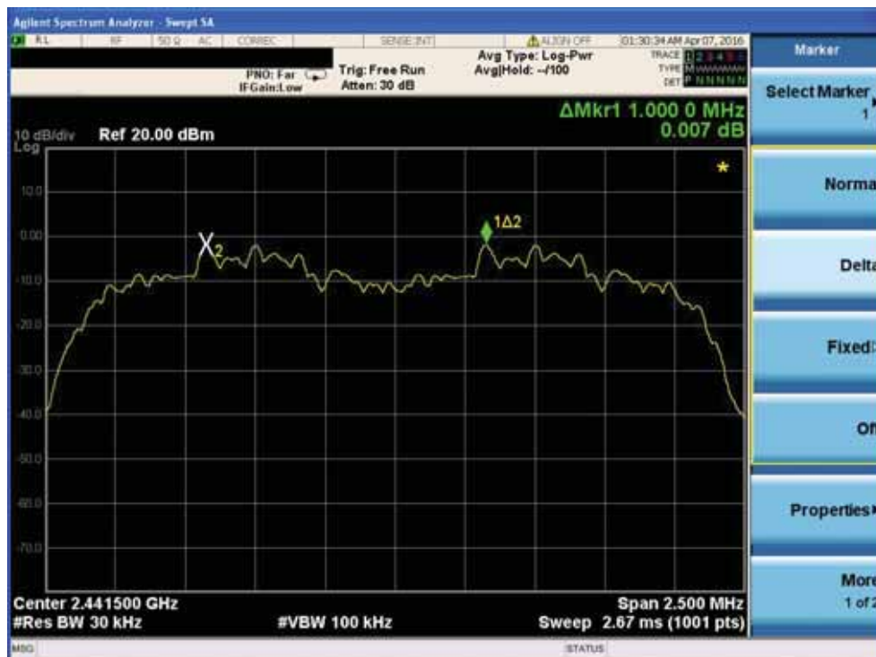
Channel Separation plot on channel 39-40
