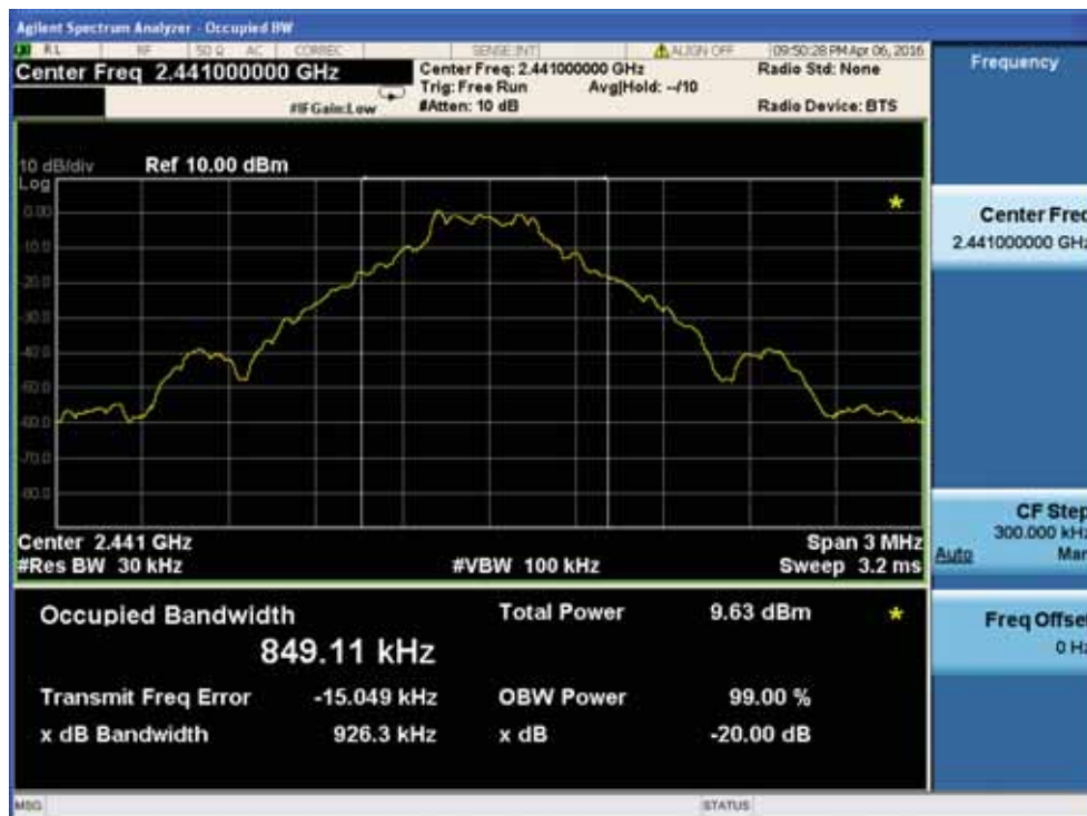
20dB Bandwidth plot on channel 39
