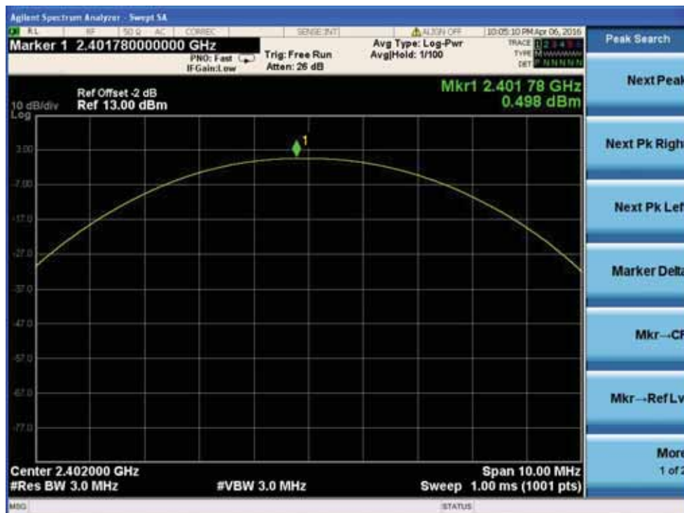
Peak output Power plot on channel 00
