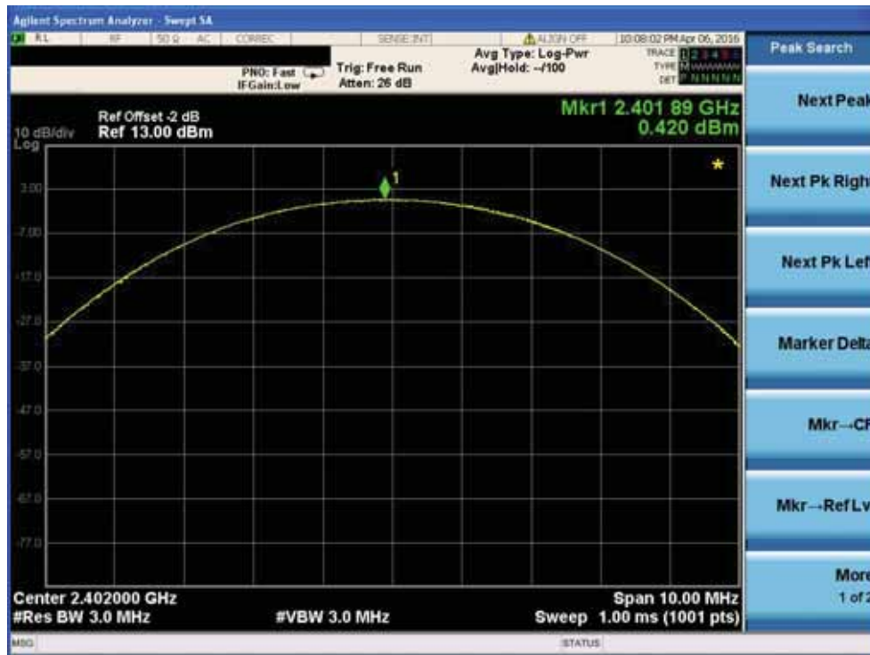
Peak output Power plot on channel 39
