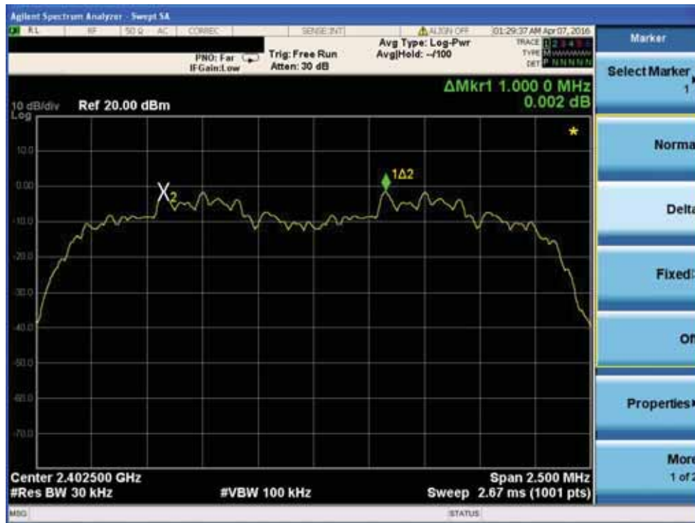
Channel Separation plot on channel 39-40
