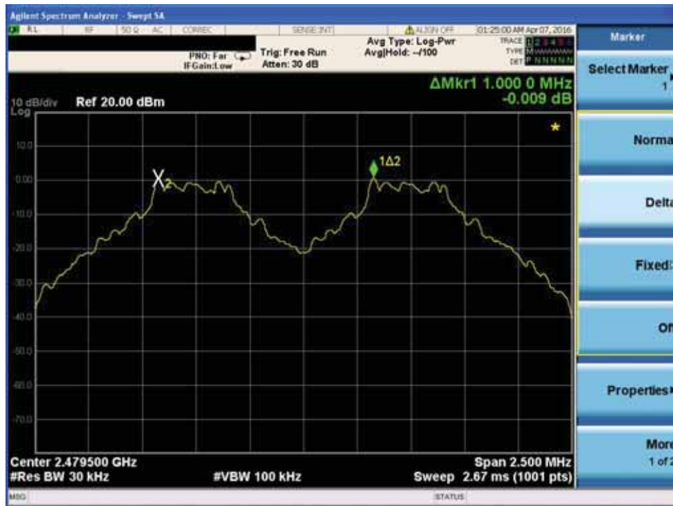
Channel Separation plot on channel 00-01
