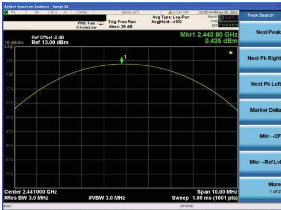
Peak output Power plot on channel 78
