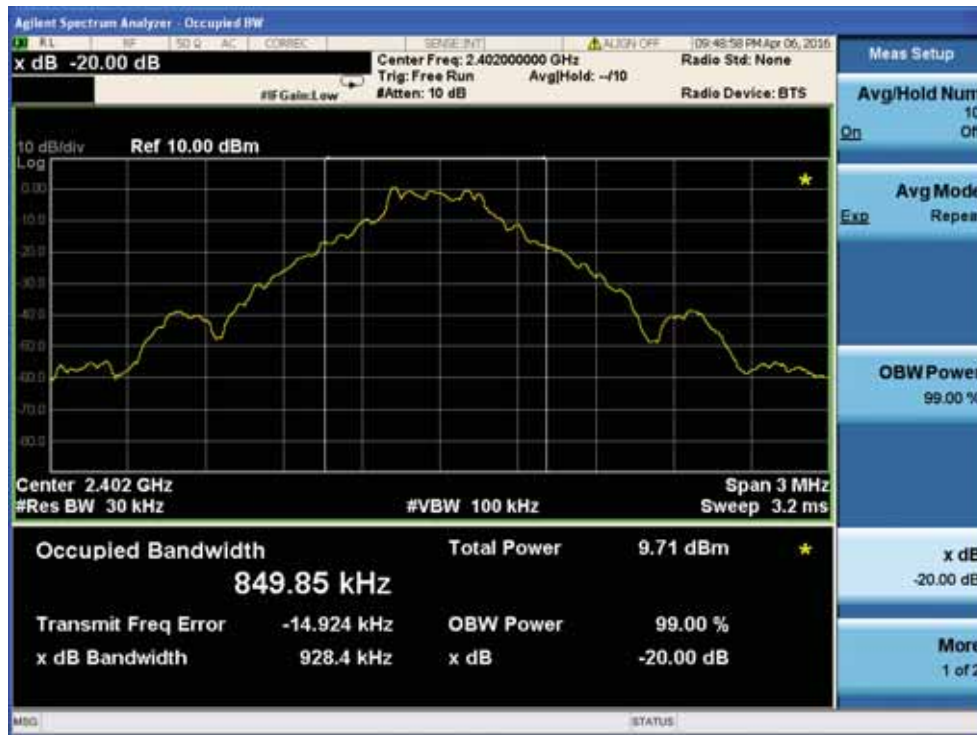
20dB Bandwidth plot on channel 39
