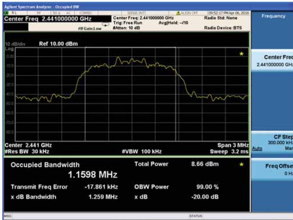
20dB Bandwidth plot on channel 78
