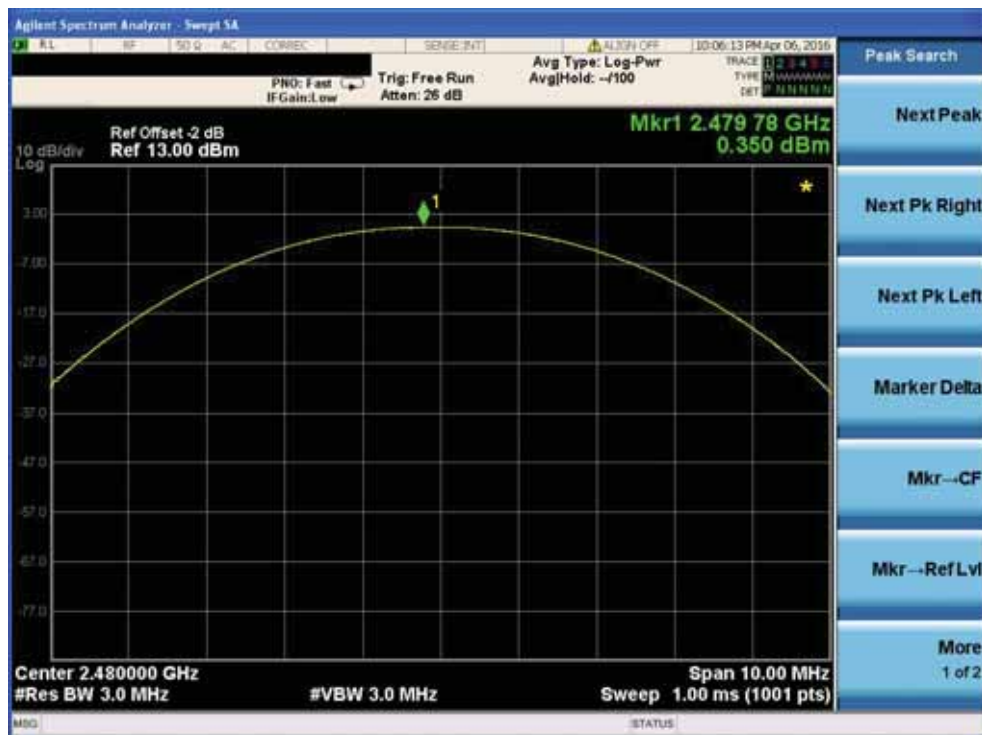
Peak output Power plot on channel 78
