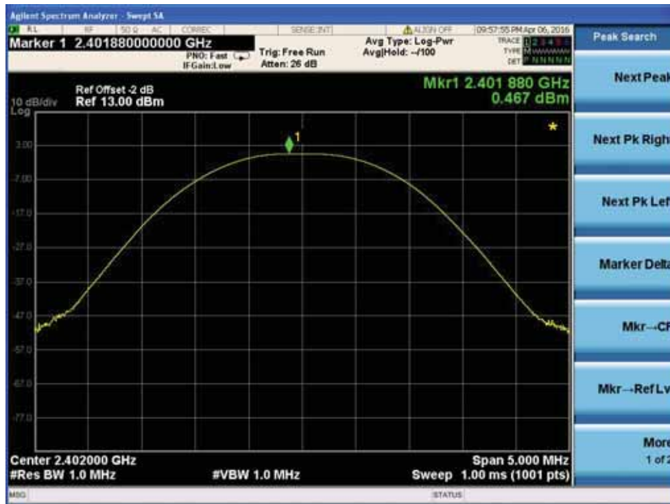
Peak output Power plot on channel 39
