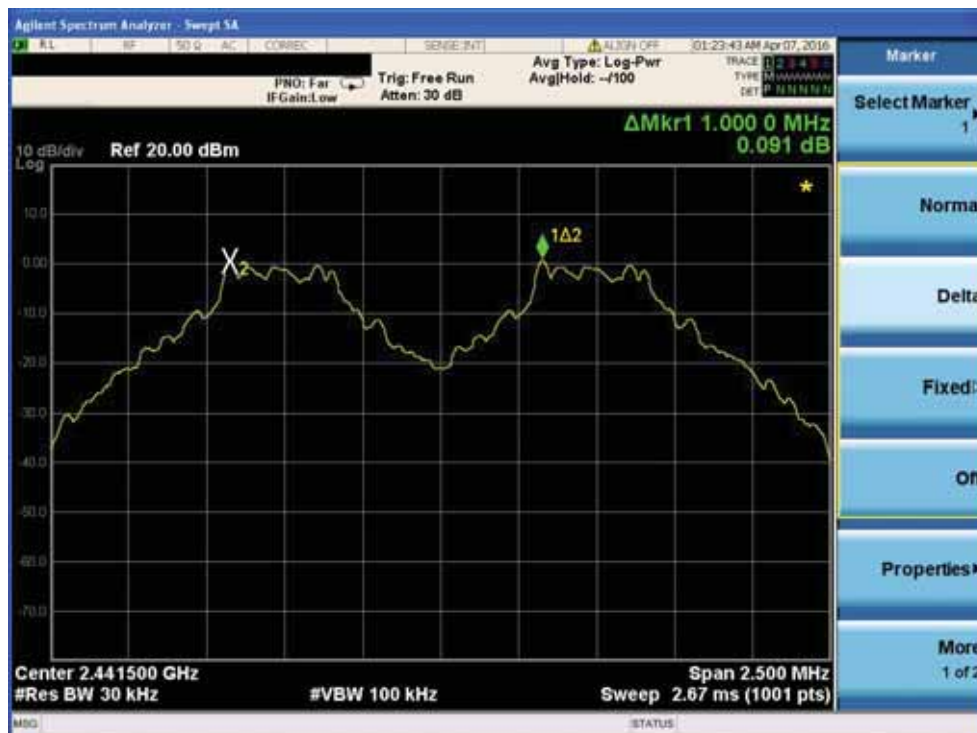
Channel Separation plot on channel 39-40
