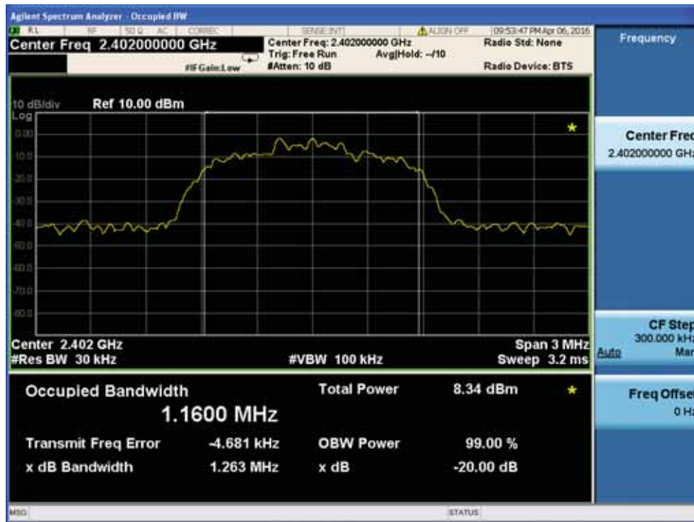
20dB Bandwidth plot on channel 39
