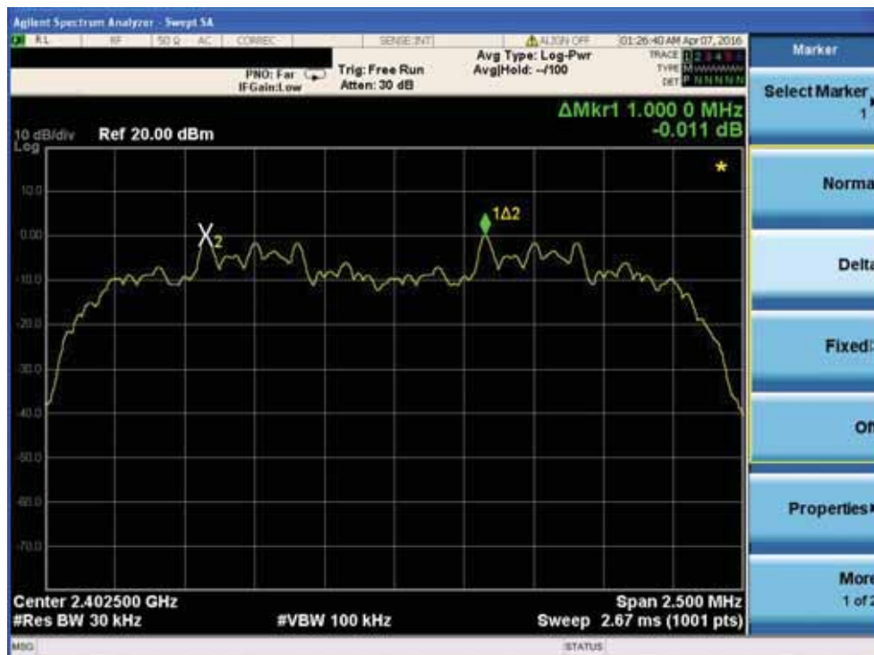
Channel Separation plot on channel 00-01
