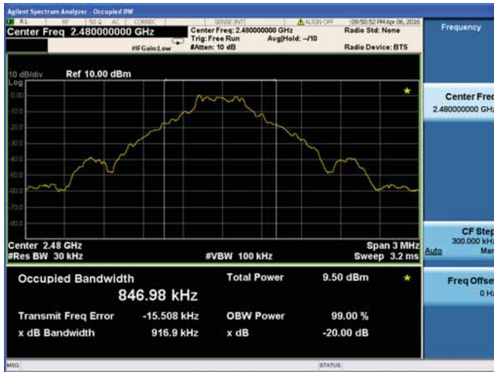
20dB Bandwidth plot on channel 00
