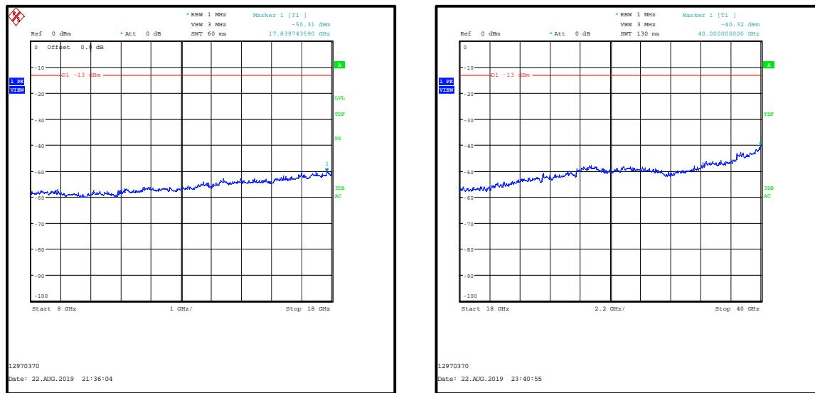
**Transmitter Out of Band Radiated Emissions (LTE Band 13 & 5 GHz WLAN) (continued)****Test Equipment Used:**
