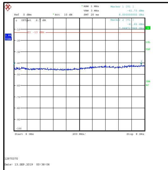
**Transmitter Out of Band Radiated Emissions (UMTS Band 4 & 5 GHz WLAN) (continued)**
