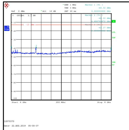
**Transmitter Out of Band Radiated Emissions (LTE Band 12 & 5 GHz WLAN) (continued)**
