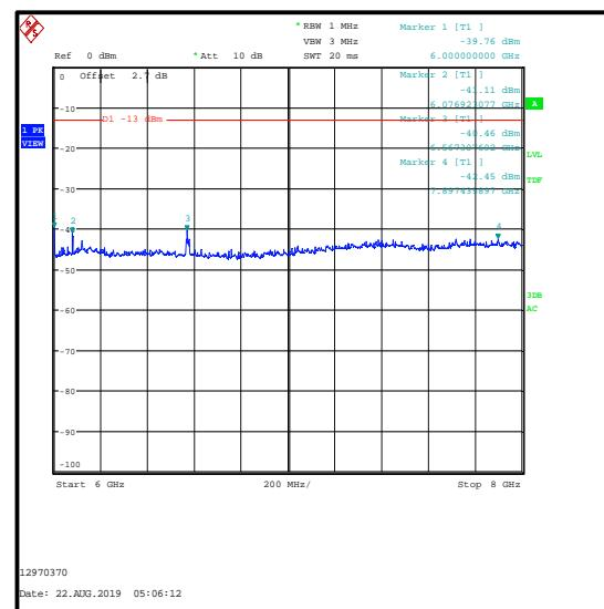
**Transmitter Out of Band Radiated Emissions (LTE Band 13 & 5 GHz WLAN) (continued)**
