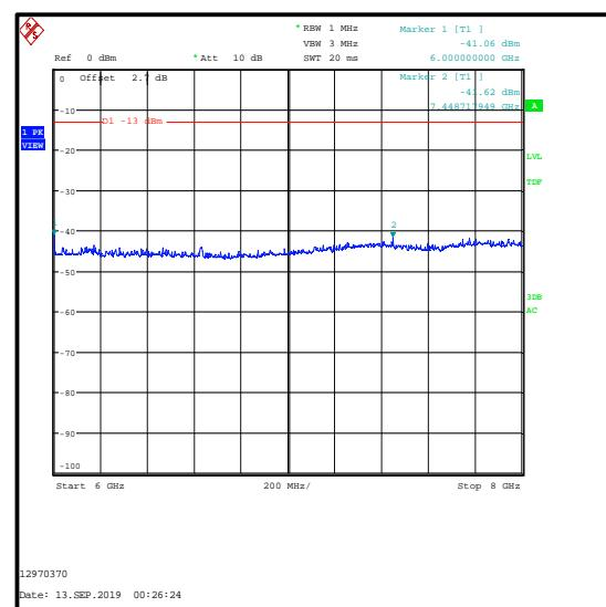
**Transmitter out of Band Radiated Emissions (UMTS Band 5 & 5 GHz WLAN) (continued)**
