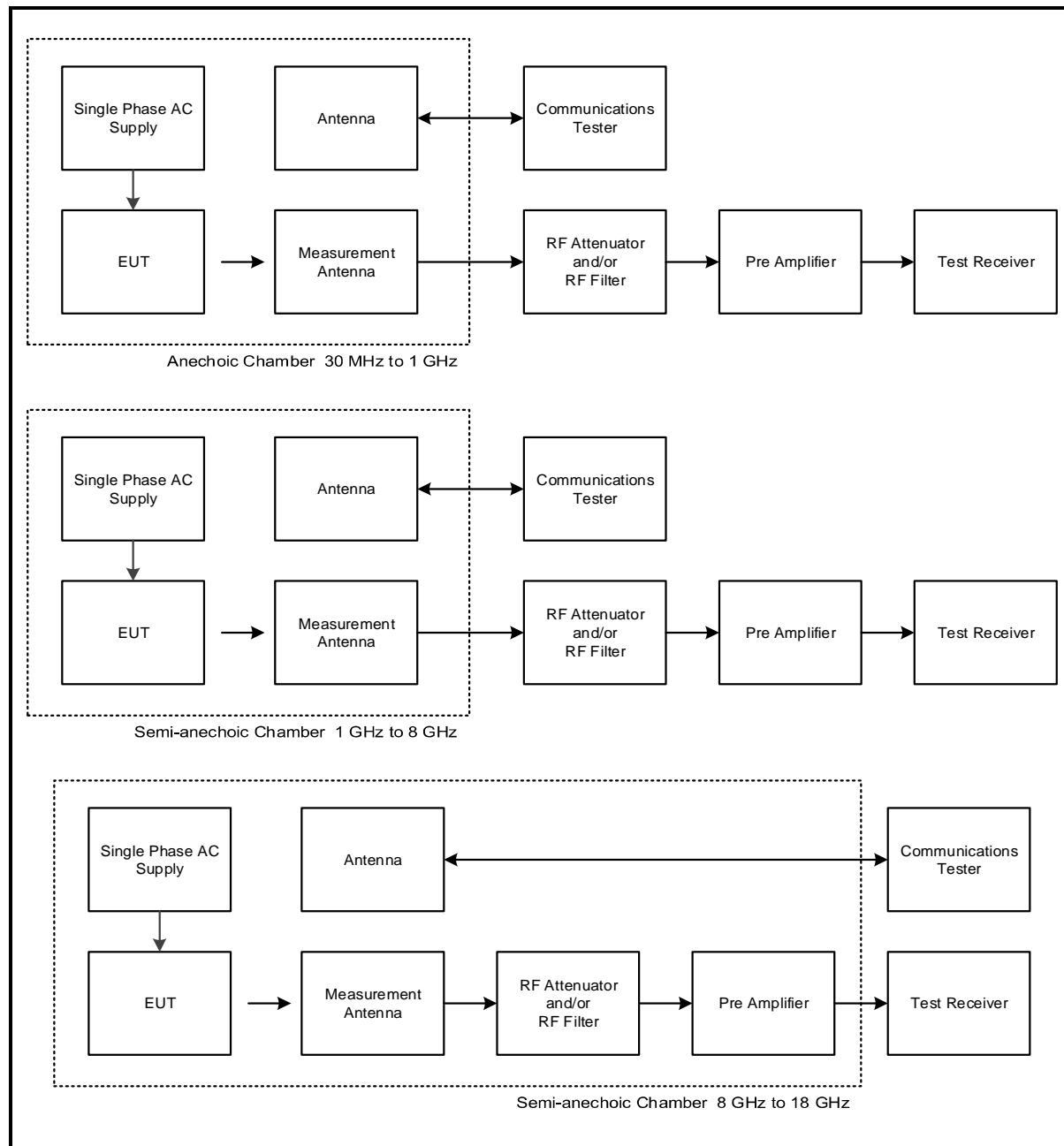
**Test Setup Diagrams (continued)****Radiated Tests:**
