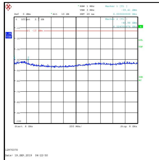
**Transmitter Out of Band Radiated Emissions (LTE Band 25 & 5 GHz WLAN) (continued)**
