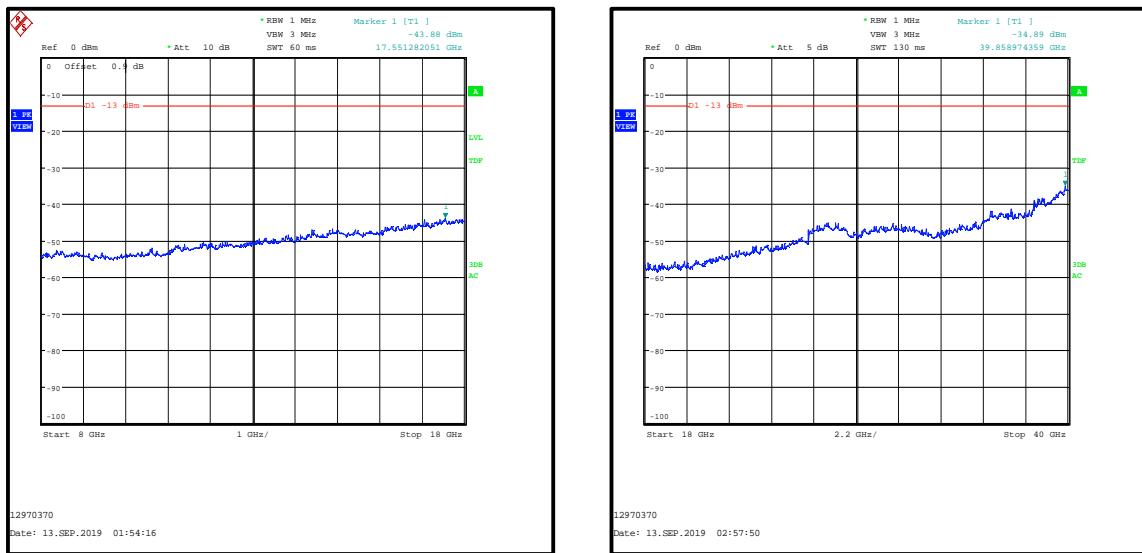
**Transmitter out of Band Radiated Emissions (UMTS Band 5 & 5 GHz WLAN) (continued)****Test Equipment Used:**
