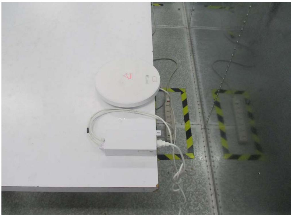
**Radiated Emission Below 1GHz Test**
