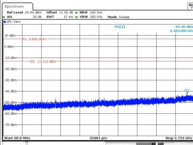
**Tx 5825MHz / 30MHz~40GHz (down 20dBc)**
