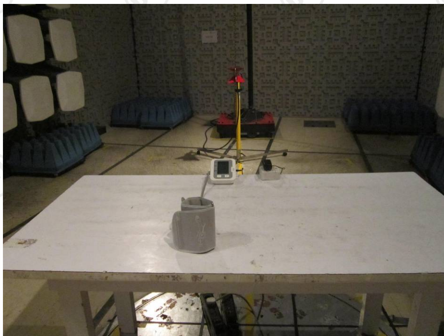
TEST SETUP OF RADIATED EMISSION-3
