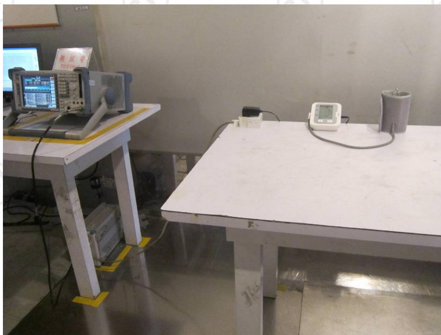
TEST SETUP OF CONDUCTED EMISSION
