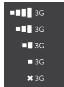
the 3G bar shows the intensity of the signal received by the camera, if no network is available, the camera will backup your pictures internally and send them when you will be back in range.
