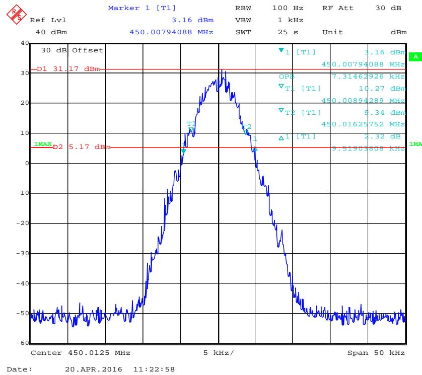
**99% Occupied Bandwidth & 26 dB Emissions Bandwidth 12.5 kHz, 450.0125 MHz (Low Power)**
