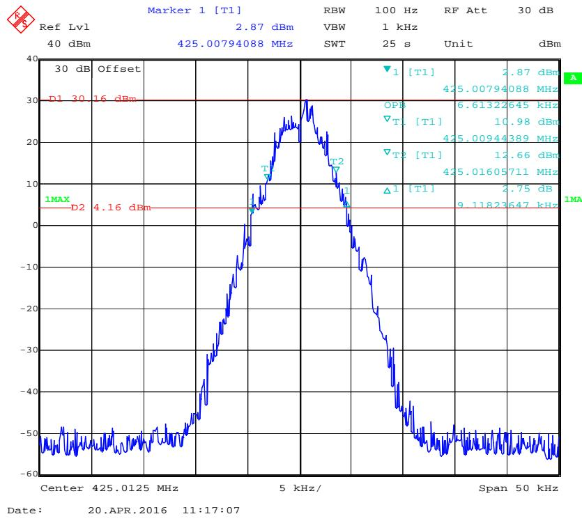
**99% Occupied Bandwidth & 26 dB Emissions Bandwidth 12.5 kHz, 425.0125 MHz (Low Power)**
