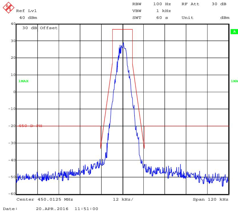
**Emission Mask D with Low Power 12.5 kHz, 450.0125 MHz**
