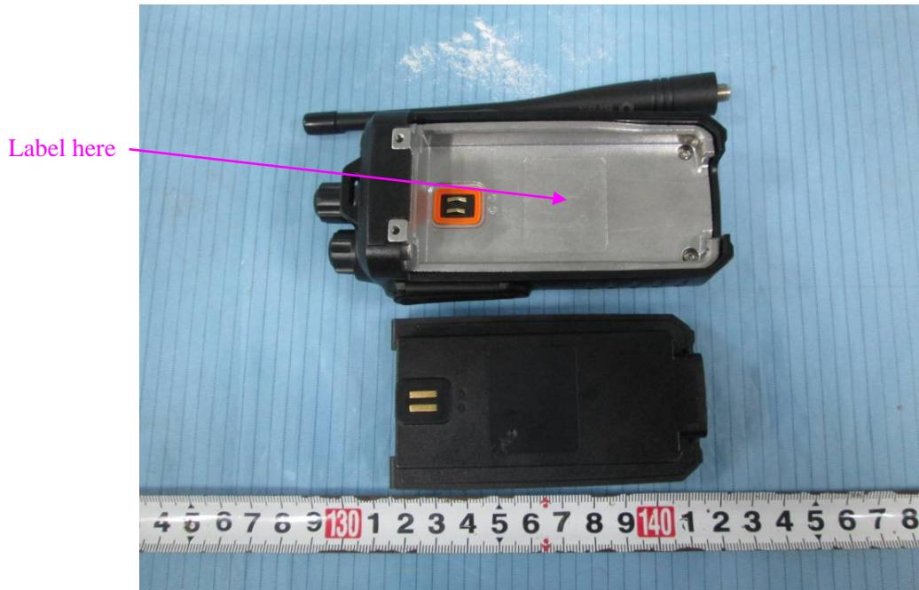
The label shown shall be permanently affixed at a conspicuous location on the device and be readily visible to the user at the time of purchase (Labeling requirements per 2.925)
