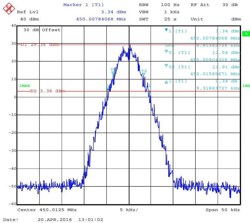
**99% Occupied Bandwidth & 26 dB Emissions Bandwidth 12.5 kHz, 450.0125 MHz (Low Power)**
