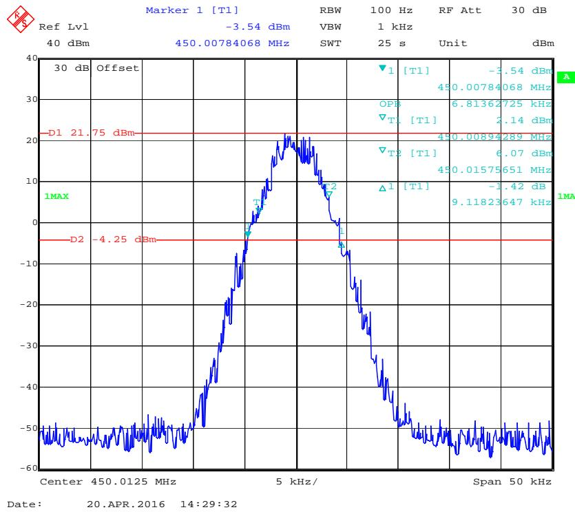
**Emission Mask D with High Power 12.5 kHz, 450.0125 MHz**
