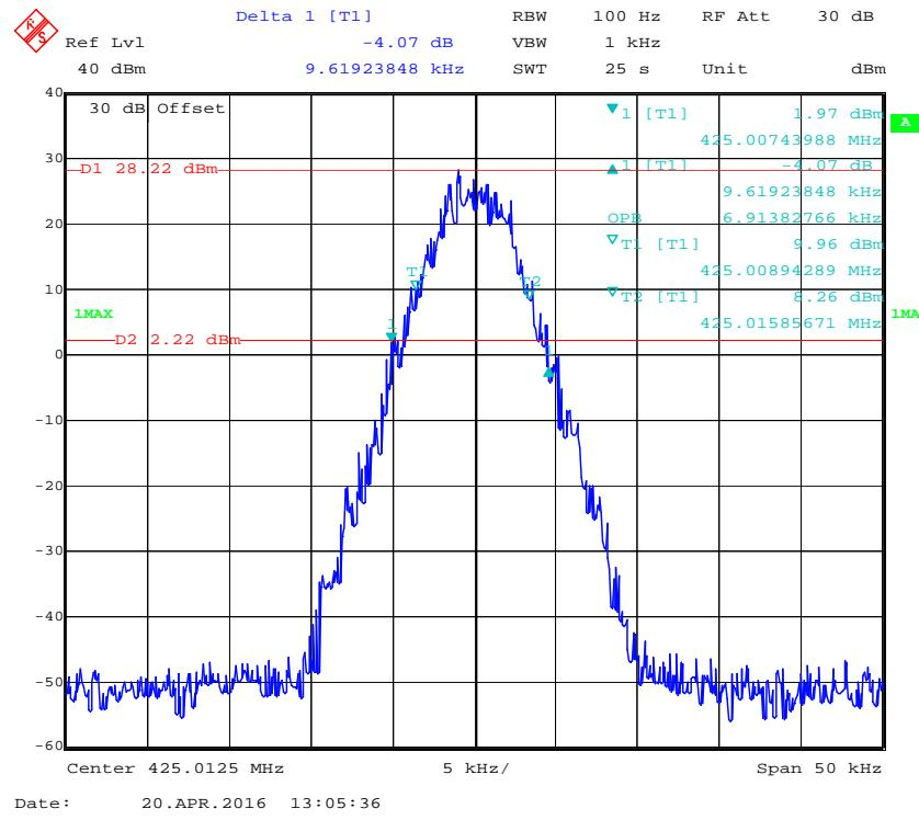
**99% Occupied Bandwidth & 26 dB Emissions Bandwidth 12.5 kHz, 425.0125 MHz (Low Power)**
