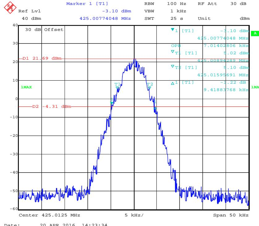
**Emission Mask D with High Power 12.5 kHz, 425.0125 MHz**
