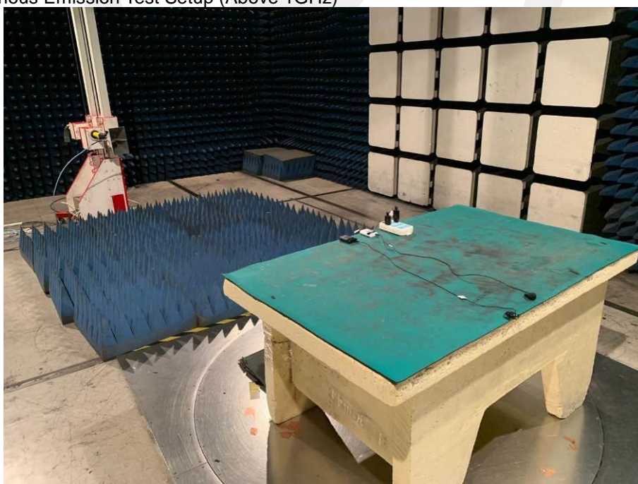
Spurious Emission Test Setup (Above 1GHz)
