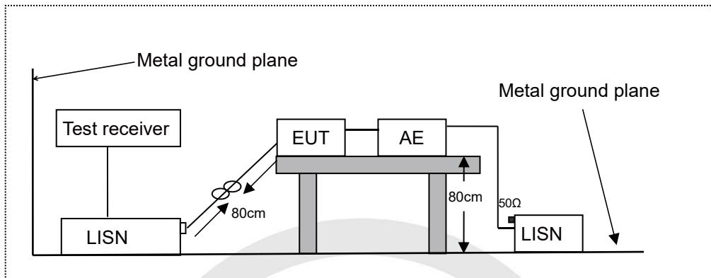
LISN: Line Impedance Stabilization Network
