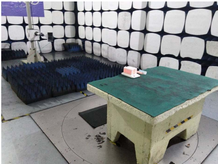
Spurious Emission Test Setup (Above 1GHz)
