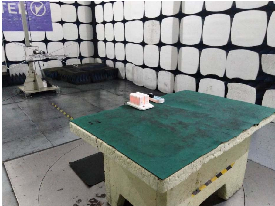
Spurious Emission Test Setup (Below 1GHz)
