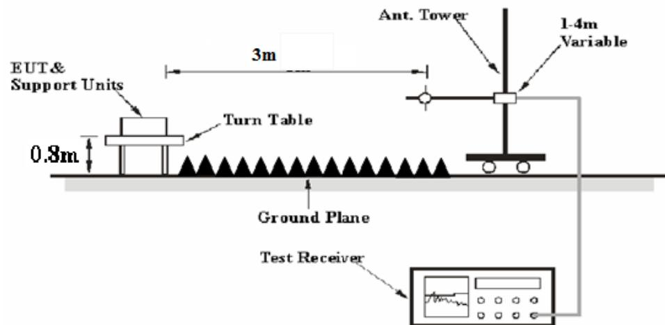
The radiated emission below 1GHz tests were performed in the 10 meters chamber test site, above 1GHz tests were performed in the 3 meters chamber test site B, using the setup accordance with the ANSI C63.4-2014. The specification used was the FCC Part 15.109 Class B limits.
