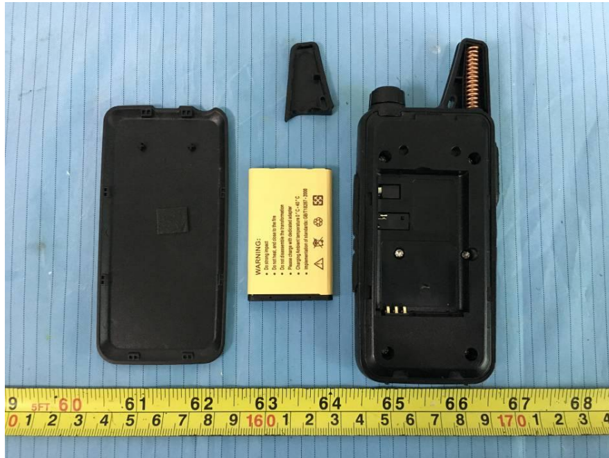
EUT – Cover off View 1
