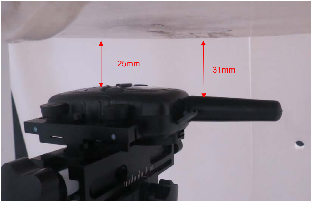
Picture 4: Face-held, the front of the EUT towards phantom, the distance from the EUT Antenna to the bottom of the Phantom is 31mm
