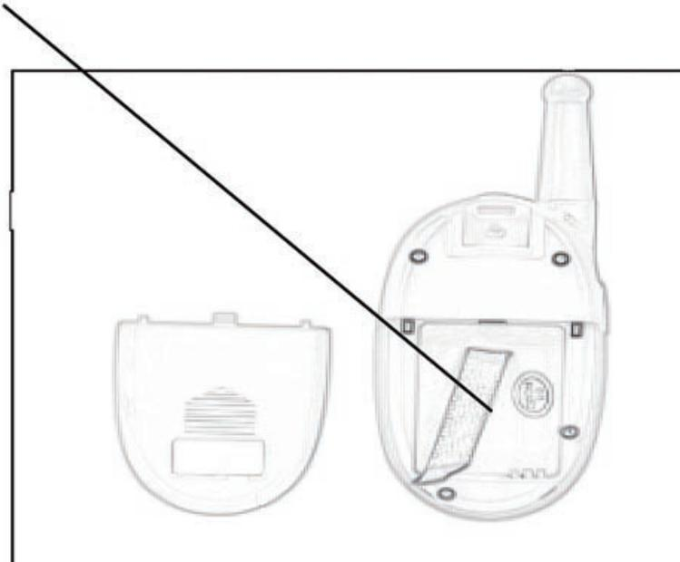
The label shown shall be permanently affixed at a conspicuous location on the device and be readily visible to the user at the time of purchase (Labeling requirements per 2.925)
