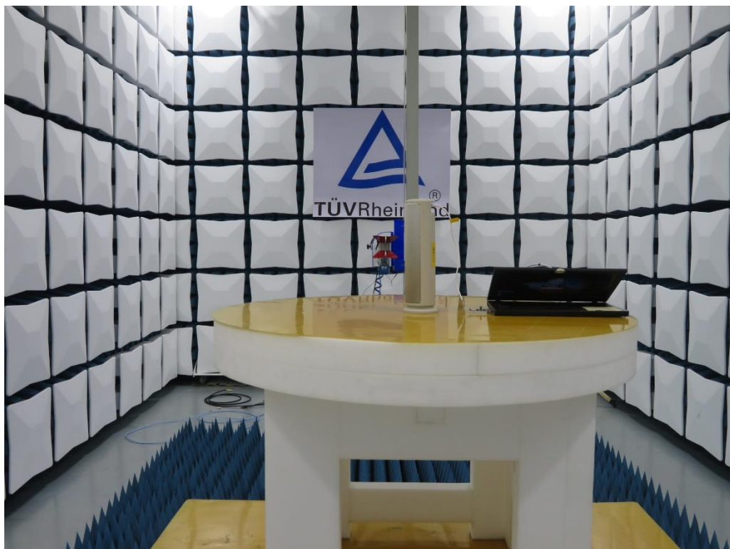
Photograph 2: Set-up for Radiated Spurious Emission, Above 1GHz
