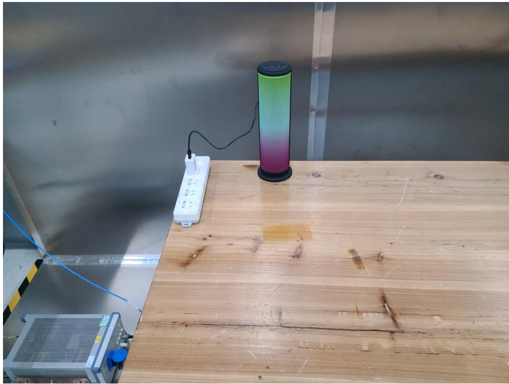
Photograph 3: Set-up for Conducted Emission on AC Mains
