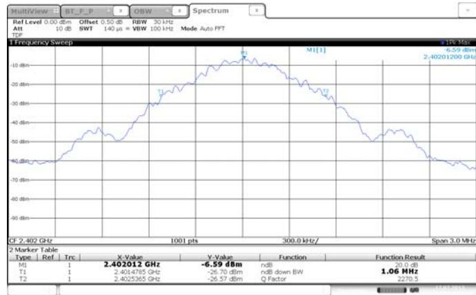
Figure 3. Plot of the 20dB Channel Bandwidth (Conducted)
