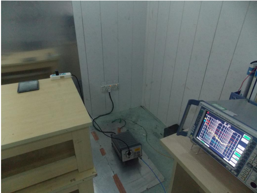
FCC RADIATED EMISSION TEST SETUP
