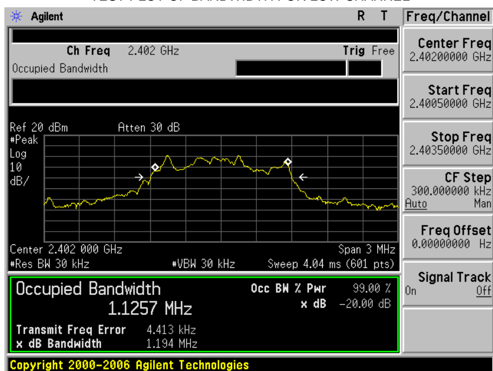
TEST PLOT OF BANDWIDTH FOR LOW CHANNEL
