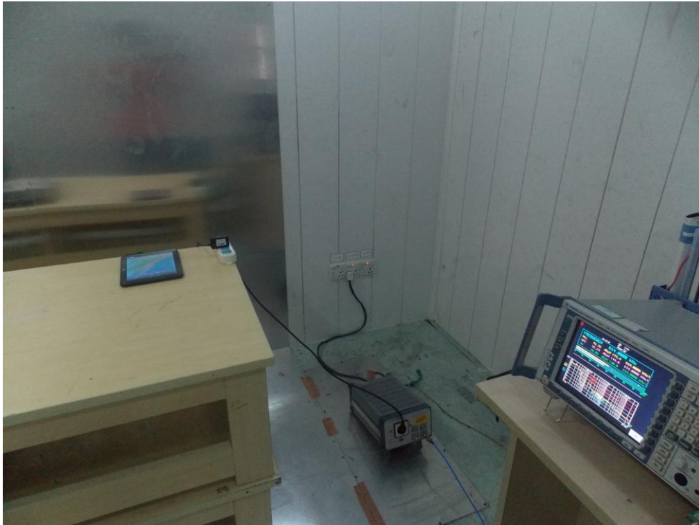
FCC RADIATED EMISSION TEST SETUP
