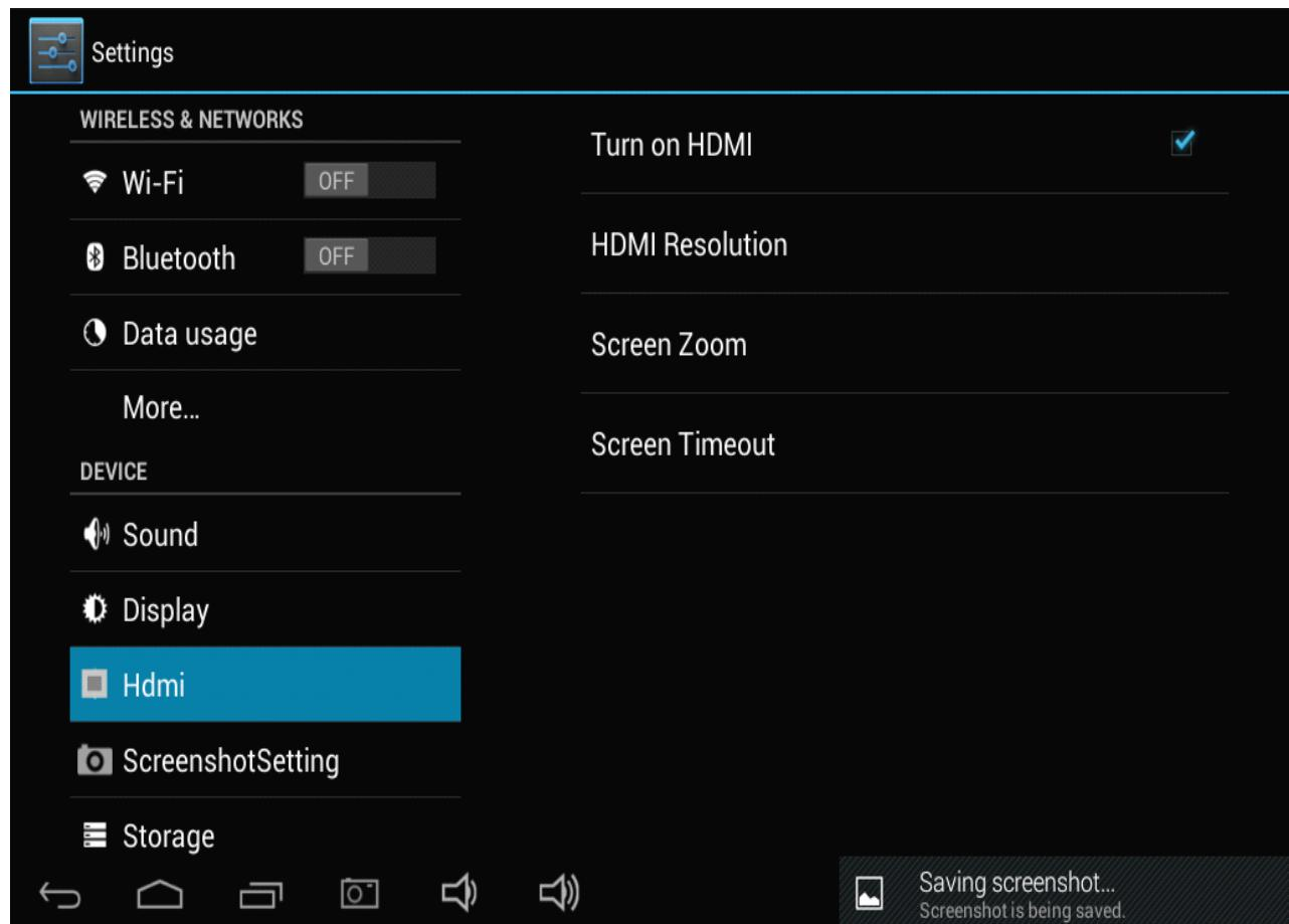
Select the option “Turn on HDMI”, then connect your device with an HDMI cable with TV or monitor. You can set the HDMI resolution and timeout in the HDMI interface.
