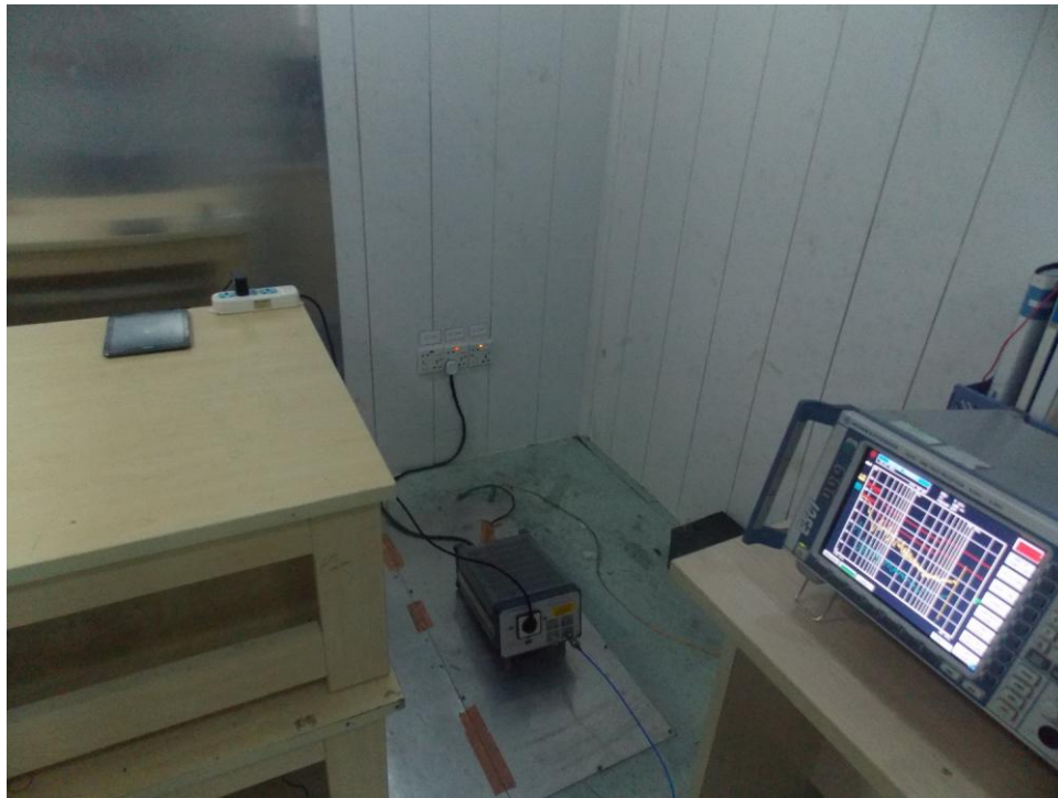
FCC RADIATED EMISSION TEST SETUP
