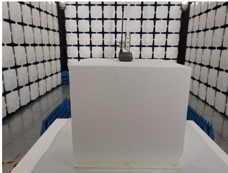
Above 1GHz for radiated emission test setup
