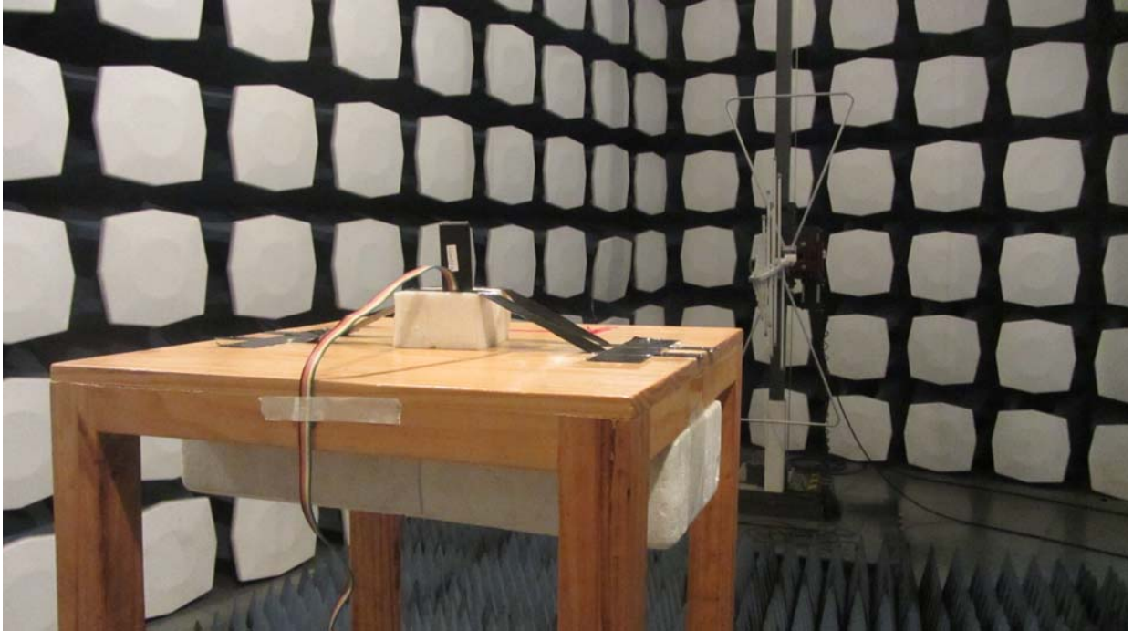
Picture 2: Radiated Spurious Emissions Test setup
