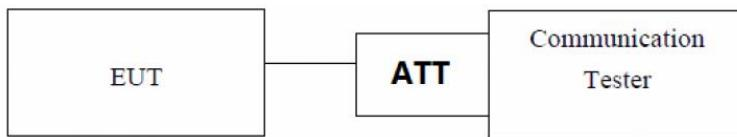
*Note: Measurement setup for testing on Antenna connector*
