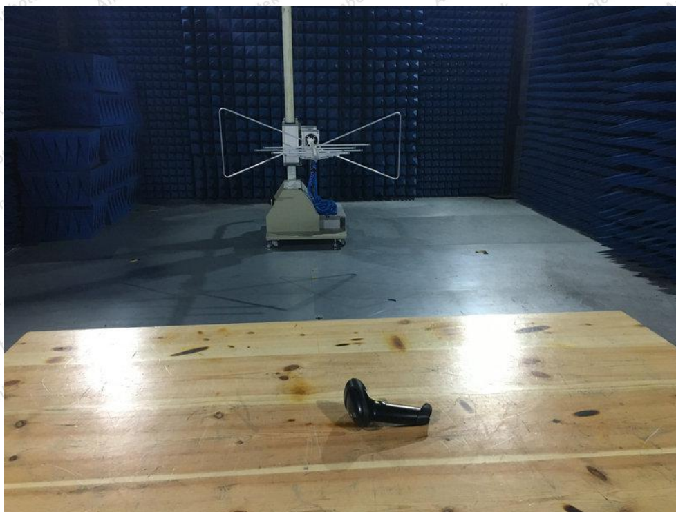
Photo of Radiation Emission Test
