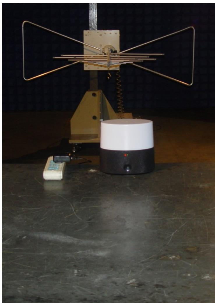
**Radiated emissions test > 1GHz**
