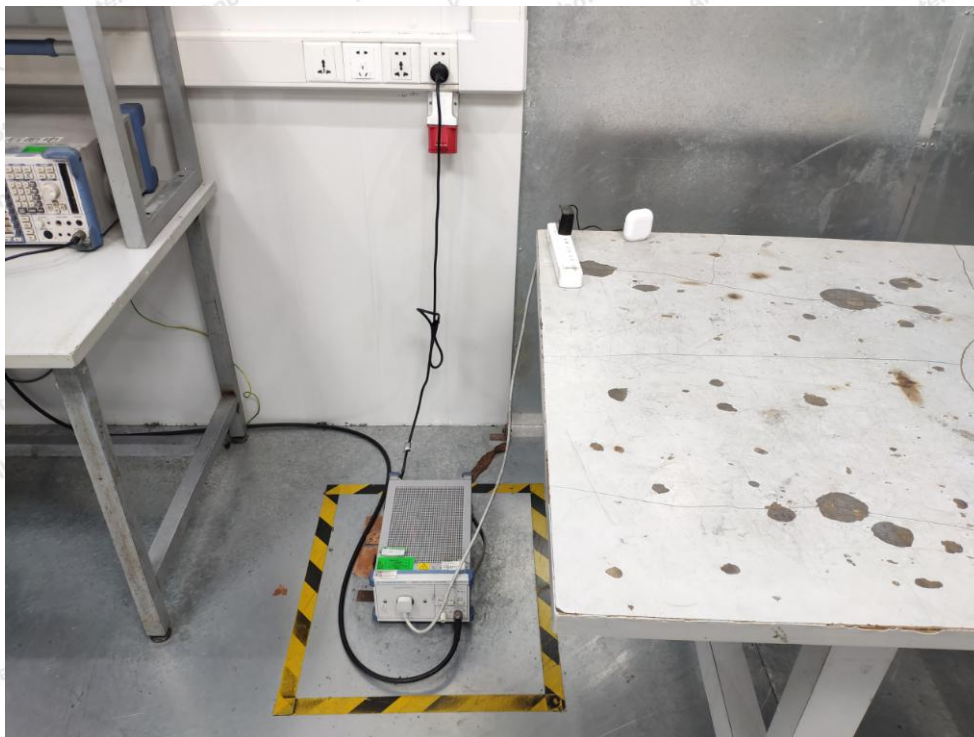
Photo of Conducted Emission Measurement
