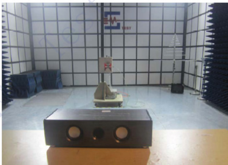
Radiation Emission Test Setup (Above 1GHz)
