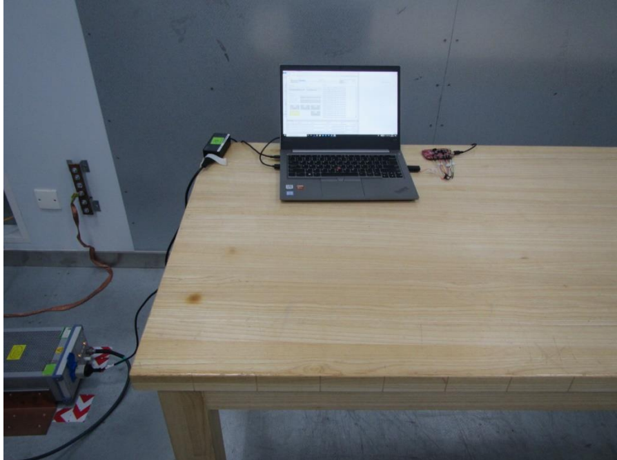
POWERLINE CONDUCTED EMISSIONS MEASUREMENT SETUP
