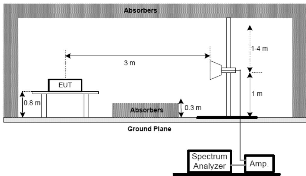
(C) For Radiated Emission Below 30MHz
