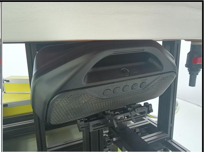
Top Side of EUT with 0 cm Gap
