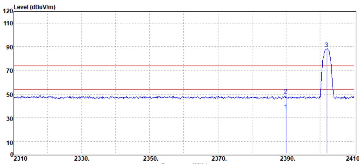
The plot shows the Level (dBuV/m) on the Y-axis (0 to 120) versus Frequency (MHz) on the X-axis (2310 to 2410). A blue line represents the signal level, which is relatively flat around 48 dBuV/m until approximately 2390 MHz, where it rises sharply to a peak of about 90 dBuV/m (labeled 3). Two red horizontal lines indicate the test limits: a lower one at 50 dBuV/m (labeled 1) and an upper one at 74 dBuV/m (labeled 2).
