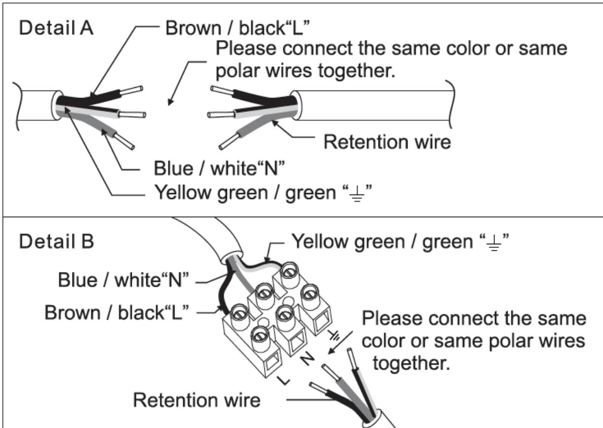
Make sure that the cables are well connected and ensure by pulling on each of them before closing all. For more security we suggest that you protect the connections with insulation tape.
