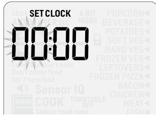
Turn TIME dial to adjust hours and press START button to confirm.
