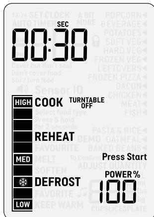
Press once again to enable the turntable to rotate again.
