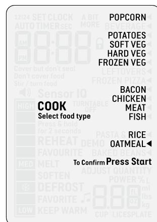
Once you have chosen FOOD TYPE, turn POWER/AMOUNT dial to adjust quantity or weight, unless Sensor IQ is being used.
