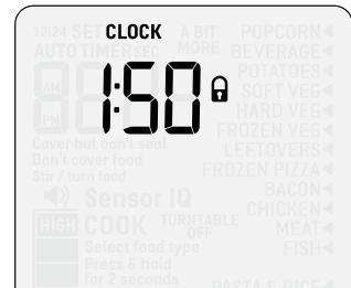
To deselect CHILD LOCK press and hold A BIT MORE button for 3 seconds.
