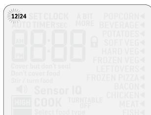
To select a 24-hour clock display, turn the START/TIME or POWER/AMOUNT dials clockwise. The number '24' will flash. Press the START button to confirm the selection.
