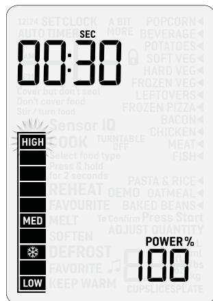
When the POWER dial is turned counterclockwise the POWER LEVEL % will start to decrease from 100% to 10%, in 10% increments.
