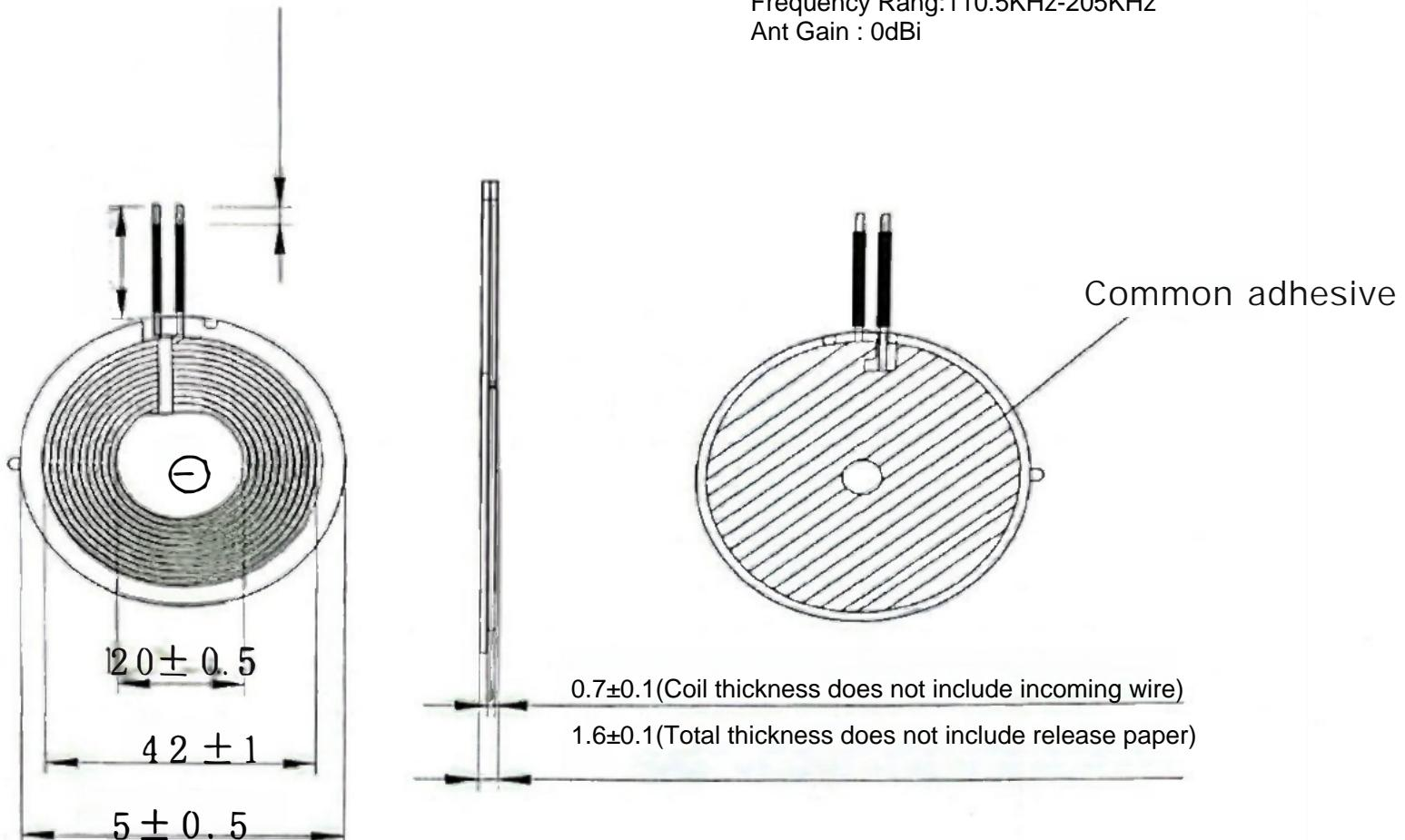
Note: The coil cannot exceed the magnetic disc
