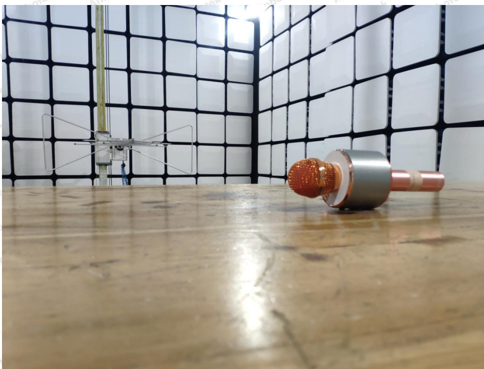
Photo of Radiation Emission Test
