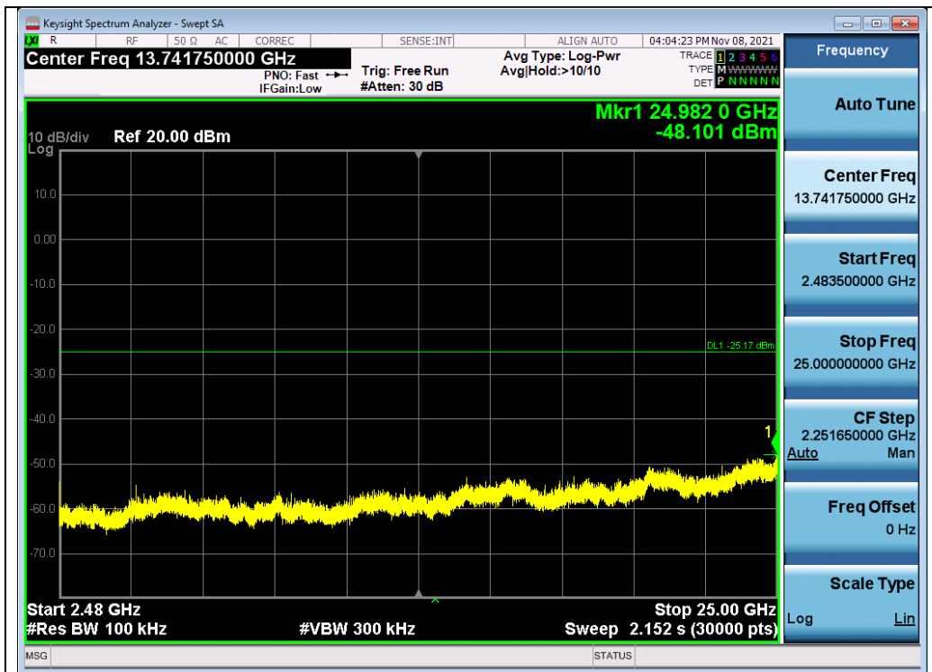
Test_Graph_EDR_ANT1_2441_2Mbps_Higher Band Emissions
