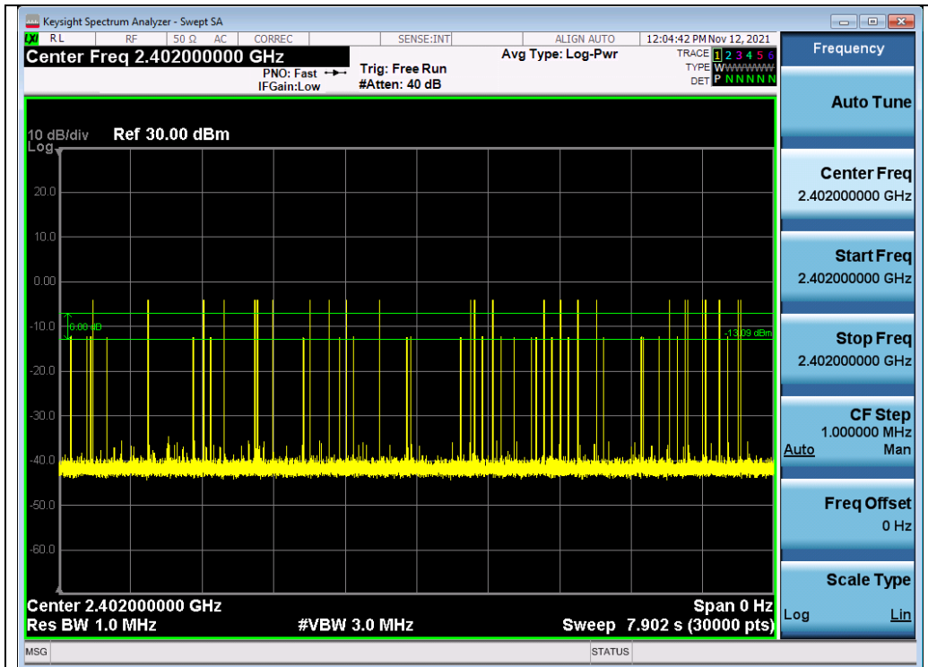
Test_Graph_BR_HOP_ANT1_NA_1Mbps_2402_Number of Burst
