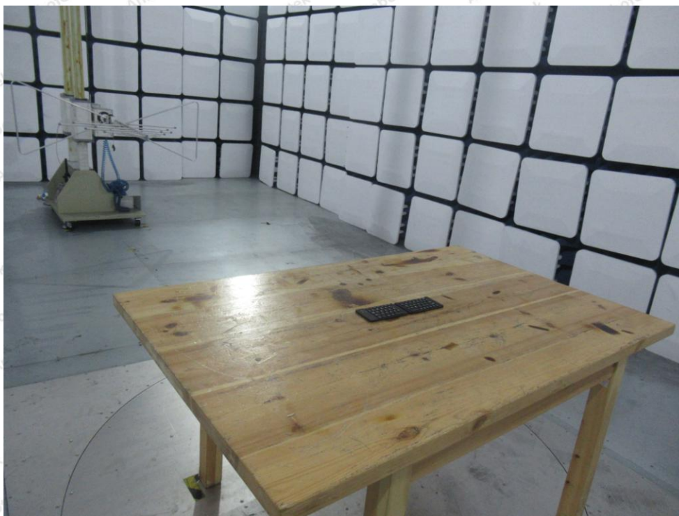
Photo of Radiation Emission Test
