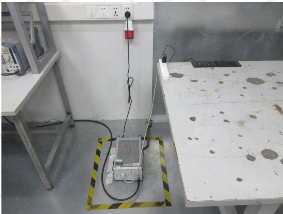
Photo of Conducted Emission Measurement
