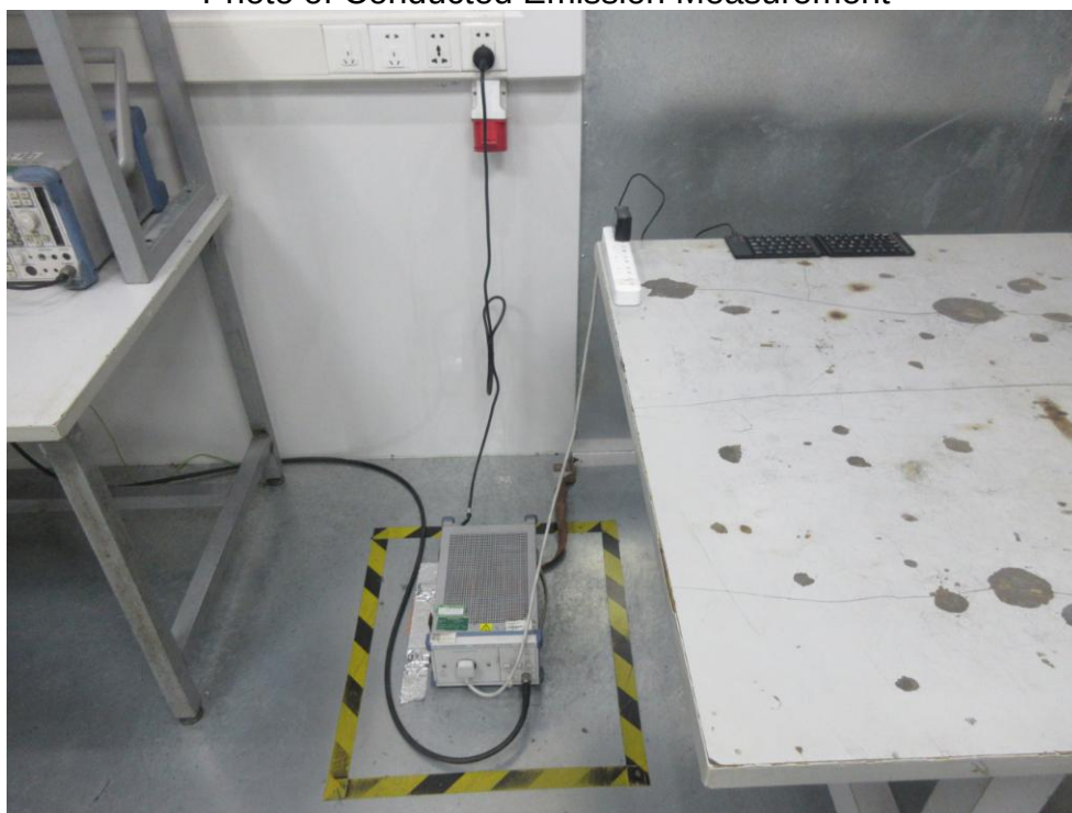
FCC ID: 2AANZFKB Photo of Conducted Emission Measurement
