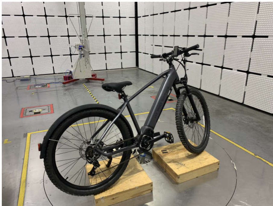
Radiated spurious emission Test Setup-1(Below 1GHz)
